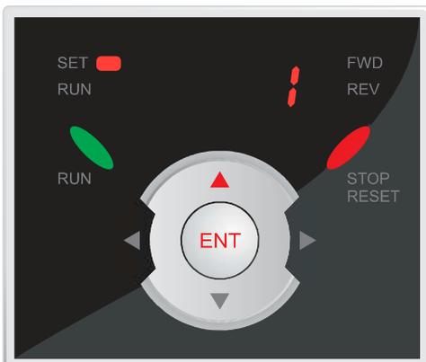
**12.3 Press the up arrow on the navigation pad to change the value from 0 to 1.**
