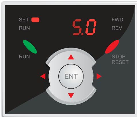
**6.4 Use the left and right arrows on the navigation pad to move between digits. Use the up and down arrows to increase or decrease the digit value.**
