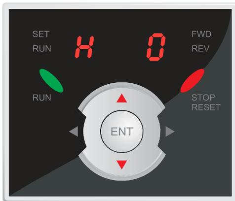
**6.2 Use the up and down arrows on the navigation pad to move between parameters within the selected parameter group.**
