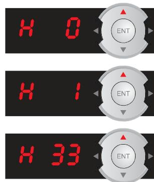
In this example, we will set Parameter H33 (Function Group 2 "H", Parameter number 33) which is motor rated current.
