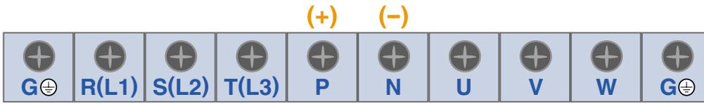
●● 22~30kW (30~40HP) <Built-in DC Reactor Type, 400V Class>
