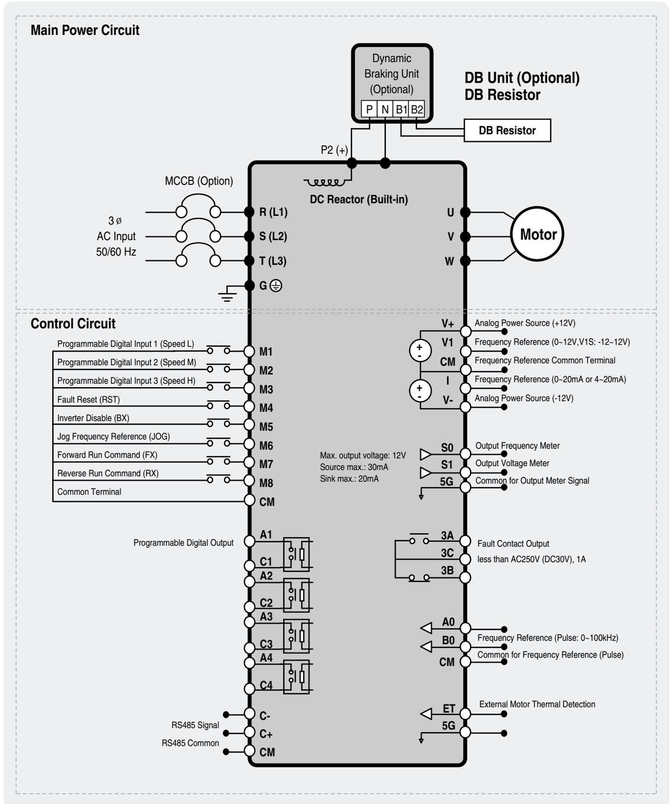
Note 1) 5G is Common Ground for Analog Meter Output (S0, S1) and External motor thermal detection (ET).
