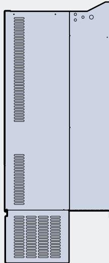
Note) Mounting NEMA 1 conduit option to the 15~90kW (20~125HP) Open Type meets NEMA 1 but does not comply with UL Enclosed Type 1. To that end, please purchase UL Type 1 product.
