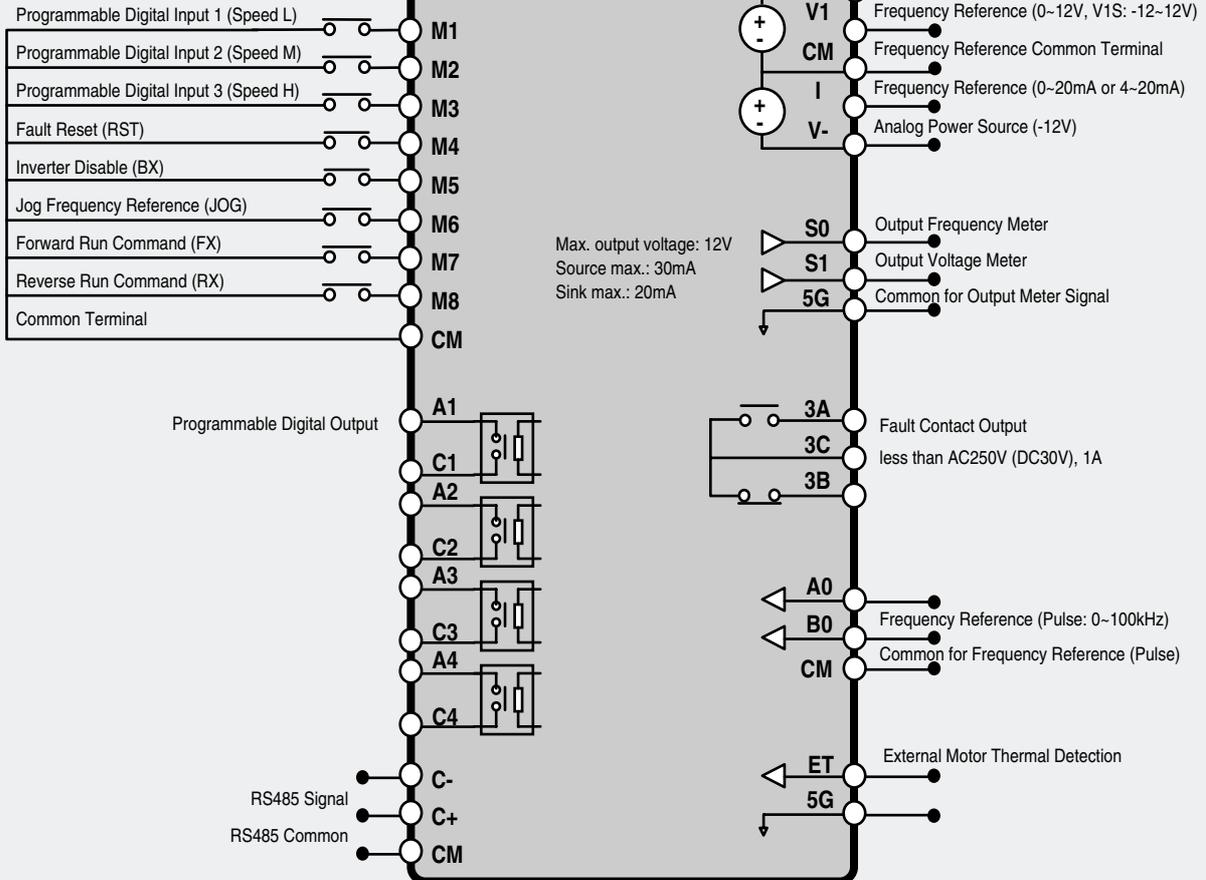
Note 1) 5G is Common Ground for Analog Meter Output (S0, S1) and External motor thermal detection (ET).
