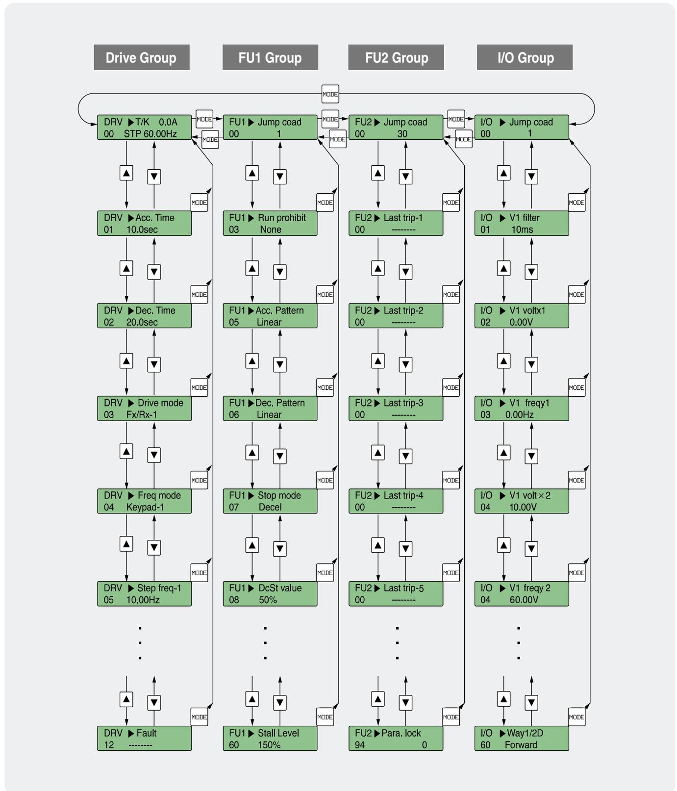
Note) This figure shows group and code navigation through LCD display keypad. It can be different from actual display due to the group addition or code change.
