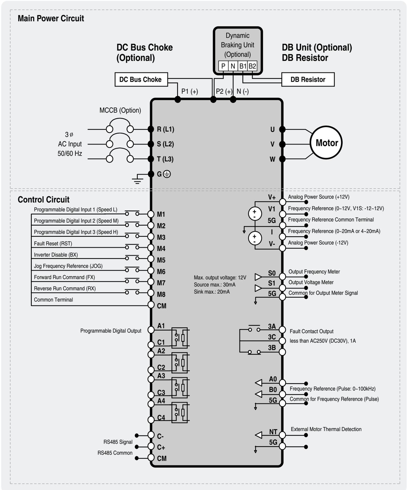
Note 1) 5G is Common Ground for Analog Input / Output.
