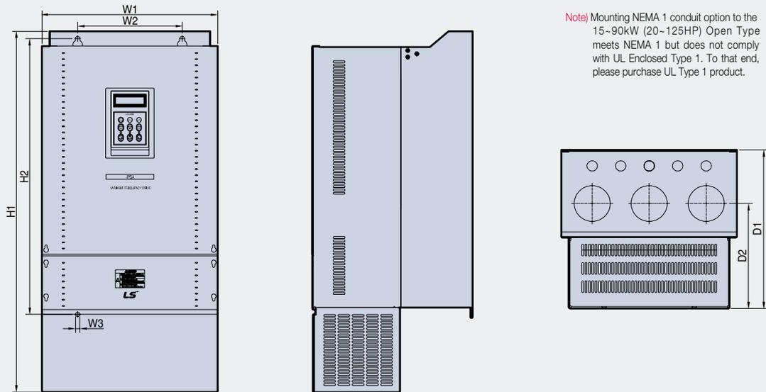
Note) Mounting NEMA 1 conduit option to the 15-90kW (20-125HP) Open Type meets NEMA 1 but does not comply with UL Enclosed Type 1. To that end, please purchase UL Type 1 product.
