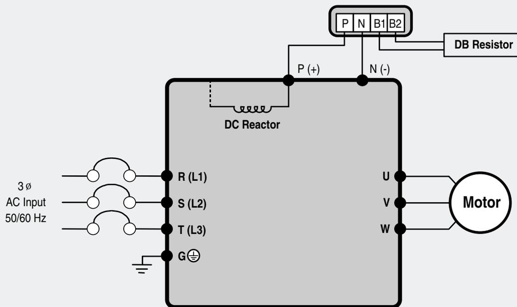
•• For 37~90kW (50~125HP) Built-in DCL Type
