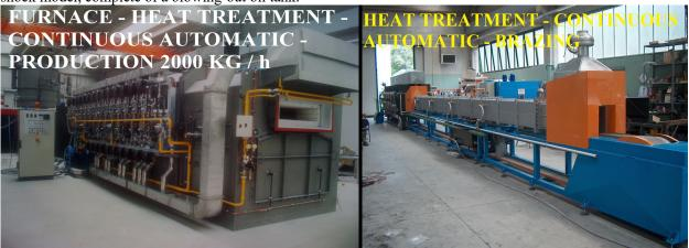
We can supply models for production till 500 Kg/h with electric or combustion feeding. The movement of pieces inside the chamber can be realized also by using a belt carrier with productions till 2000 Kg/h.
