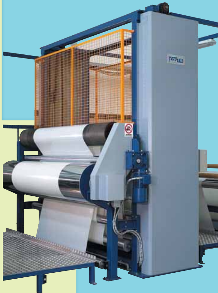
Particular of heating coating cylinder for paper
